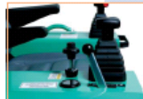
Rotor Speed Control allows the operator to set the rotor speed and reduces the amount of foot pedal travel to relieve fatigue during low speed painting.
