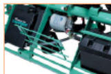
Removable panels make servicing easy by allowing quick access to filters and blowers.
